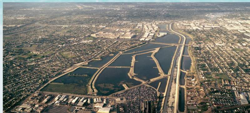
Local stormwater runoff is collected in a comprehensive set of groundwater recharge basins throughout the Region.
